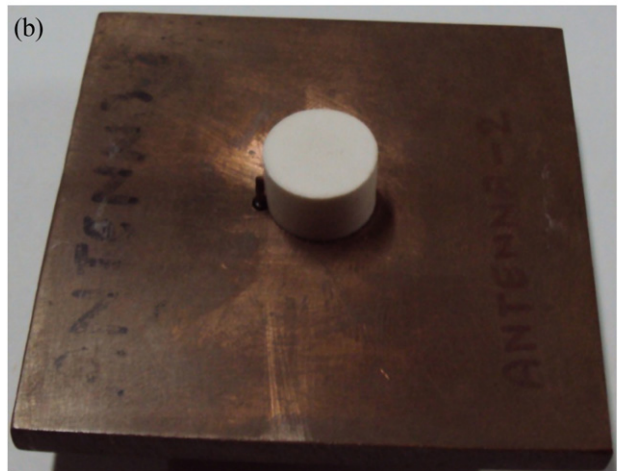
Fig. 4. Antenna geometry (a) layout and (b) fabricated structure.
